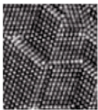
5 Atoms of silicon 1 nm
